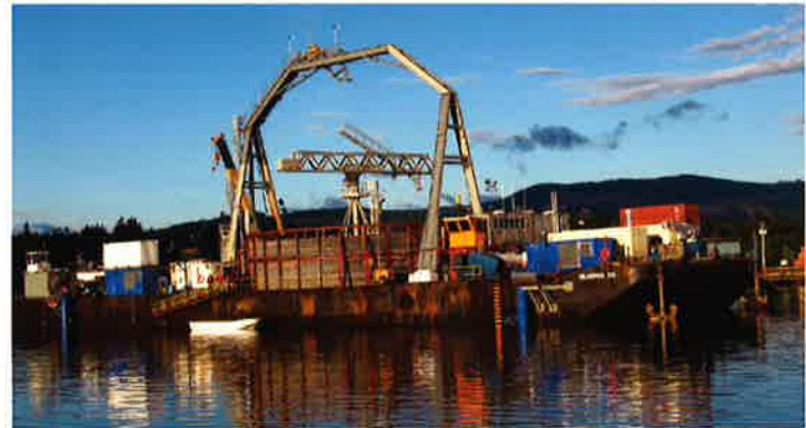
Caldwell Marine International's "Seaspan 201" DP-II Cable Lay Barge Loaded with 1600 tonnes of Cable
