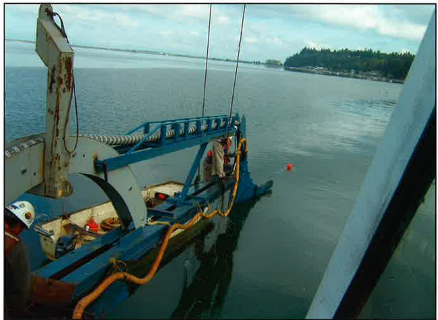
Caldwell Marine International's Low Impact Eel Grass Injector
